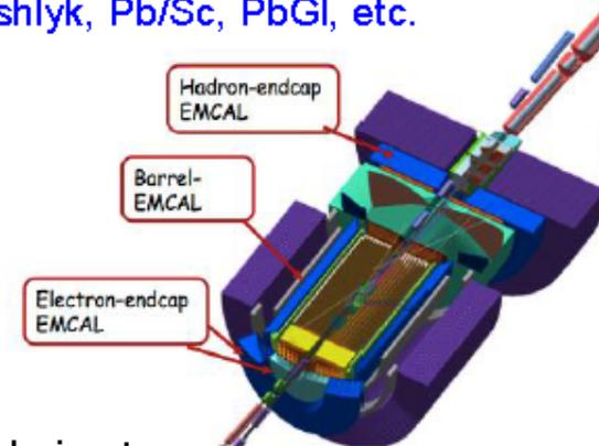
Detector Matrix for the calorimeters
