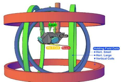
Three sets of Helmholtz coils to provide polarization in 3-d
